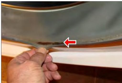
L. Picture 1 Mold-like Growth
